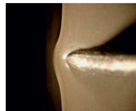
The sealing lips of a radial shaft seal, following a test cycle with a standard FKM material (above, with crack formation when lifting) and a BRE-FKM material 75 FKM 260507.
